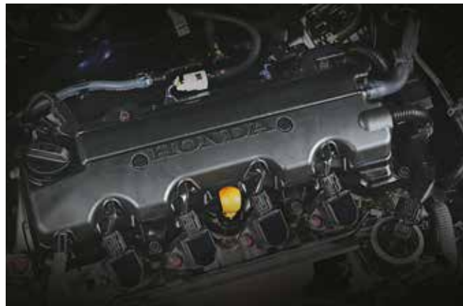
1.8L i-VTEC Engine Feel the power with fuel economy Max. Power (net): 140 ps @ 6,500 rpm
