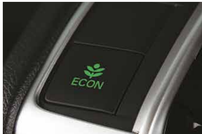
ECON Press the ECON Button to adjust vital system that effects fuel economy such as throttle, shift maping and air conditioning
