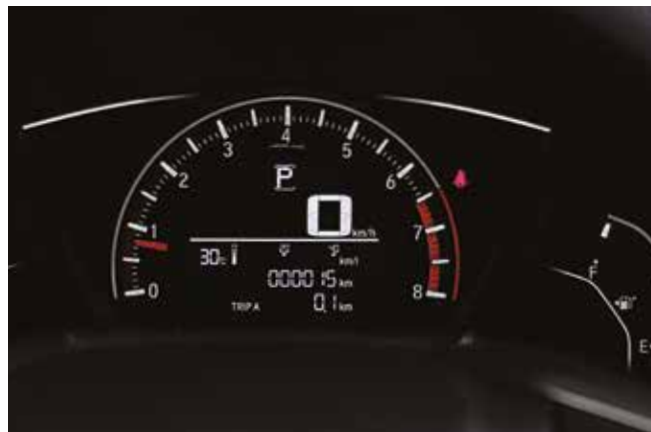
ECO Coaching The multicolour display indicator helps you to monitor your driving style and gives you real-time updates so you can drive as economically as possible
